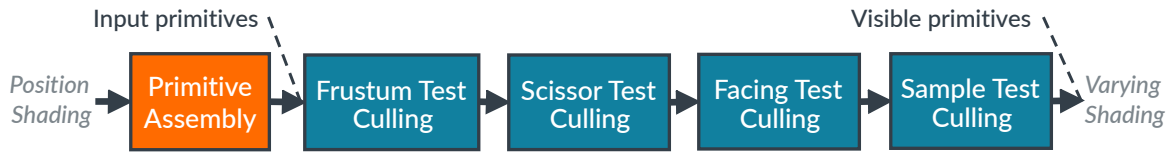
Figure 4-1: Arm GPU Gen5 GPU culling pipeline
